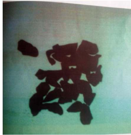
Plate 2: Sample of Solid by-product (bio-char) after torrefaction process
